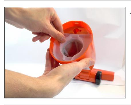
Slot the new dust cup back into the cavity.
