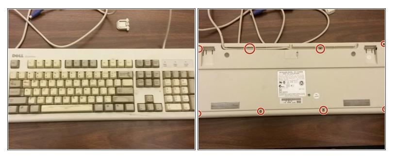
Turn the keyboard over onto its back and remove the eight Phillips #2 screws.
