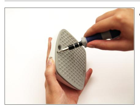
Use the screwdriver to remove the lone screw.
