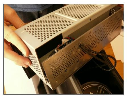
Remove the portion of the metal housing that you freed with the 7 screws in the previous step.
