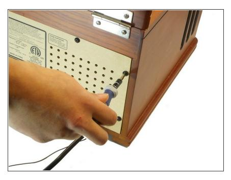
Using your Phillips head screwdriver, remove the 10 outer black screws from the back of the device.
