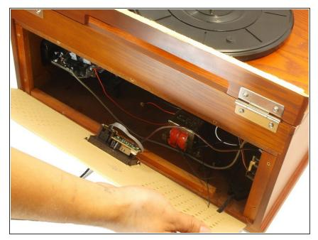
Gently remove the back of the device, being careful not to pull any wires out of place.
