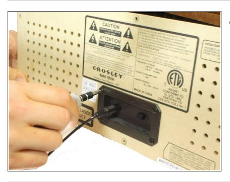
Using the Philips head screwdriver, remove the 4 black screws from the audio input box.
