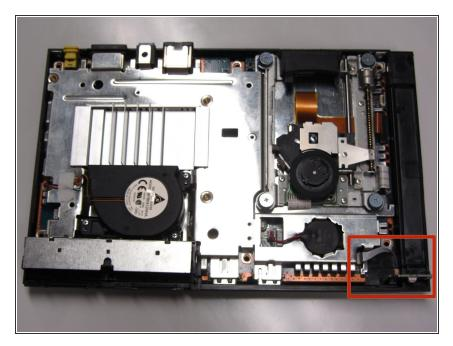
Locate the IR sensor at the front, right corner of the unit.
