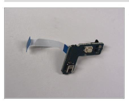
Gently lift and remove the IR Sensor from its designated slot.
