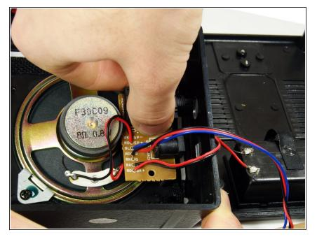
Grab the headphone jack from inside the case and pull it toward the speaker until you can fully remove it from the device.
