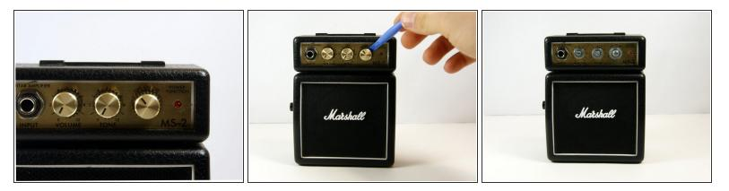
• Remove the volume, tone and power knobs by pulling them straight away from the front of the device. If they do not come off easily use the wedge tool to pry them up.
