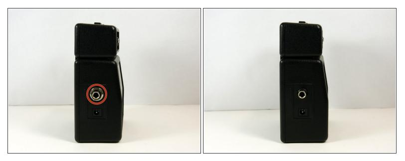
Use a 9/16" socket to remove the nut around the headphone jack. Be careful to not lose the washer.
