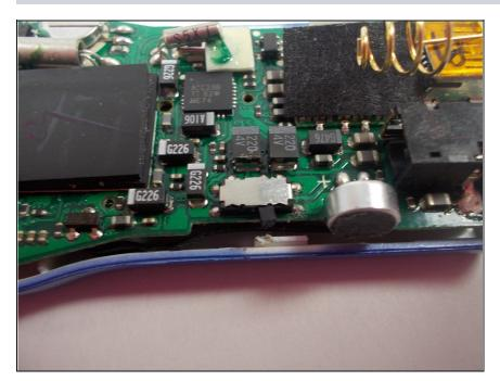
Replace the faulty hold switch with a new one.
