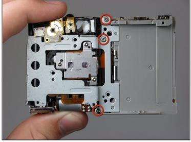
Unscrew one Phillips screws from the side and three Phillips screws from the back panel using a #0 Phillips screwdriver.
