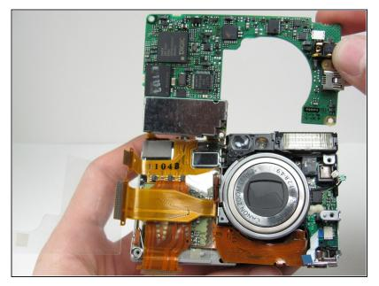
• Free the logic board from the rest of the camera.
