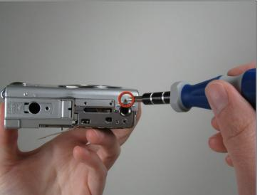
• Unscrew the four Phillips screws from the side of the casing and one screw from the bottom using a #0 Phillips screwdriver.
