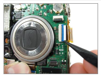
• Lift the blue ribbon gate using the Spudger.
