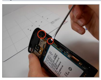
Insert a flat head screw driver under the two clips and pry up.
