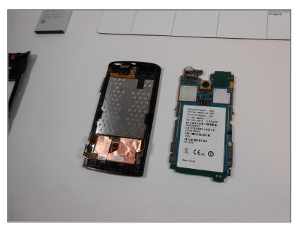
Logic board should be removed from the phone. Put it off to the side.
