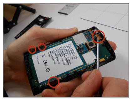
Using a flat head screw driver, undo the ribbon cables connected to the phone. There should be two on the left, one on the right, and one on the top.
