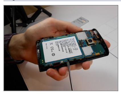
Gently insert a flat head screw driver under the logic board and pry to remove it from the phone casing. There should be a notch where a screw driver can fit as indicated in the image.
