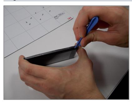
• Use a case opening tool to release clips holding together the case. It should be easier starting at the bottom right side of the phone, as indicated in the image. Insert the tool and run it down the side of the phone, using a prying motion to pull it apart.
