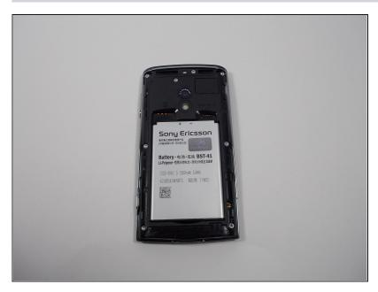
Place the phone with the back facing up. Remove the back cover and the battery.
