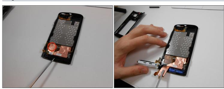
• Using a flat head screw driver, disconnect the glue holding the left ribbon cable to the phone. Once unglued, the cable should flip back and still be connected to the phone. Pull up the black plastic piece being pointed to in the image.
