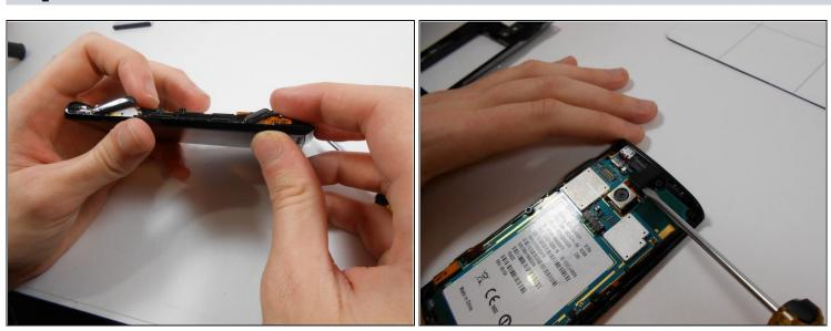
• If the volume rocker and camera button haven't fallen off yet, remove them and put them off to the side. Using your fingers or a screwdriver, pull off the black plastic piece on the very top of the phone. This is the audio jack.
