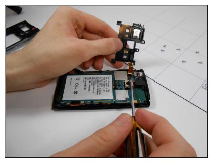
• Flip the chip to the left and remove the ribbon cable from the rest of the phone using a flat head screw driver. Gently insert the screw driver under the cable and pry up.
