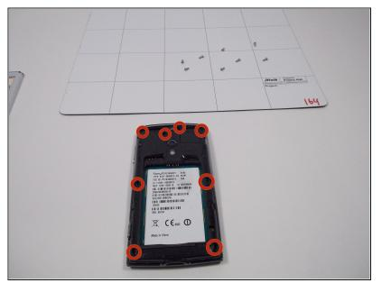
Remove the 5mm screws from back of the phone, image indicates where they are.
