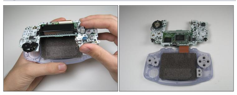
• Pull circuit board away from the front panel by pulling up at the bottom of the circuit board, keeping the top ribbon still connected.
