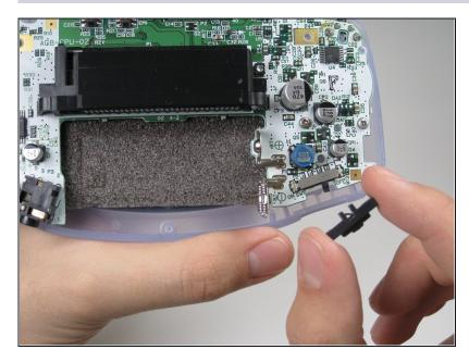
• Remove the gray **On/Off** Switch by pulling up and away from the unit. Replace with another switch if necessary.
