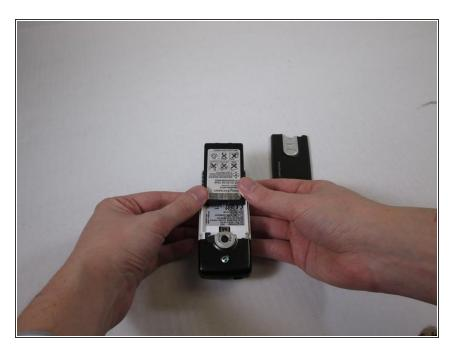
Slide the battery upward to remove.
