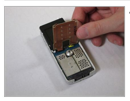
Gently lift the white circuit board to reveal the base.
