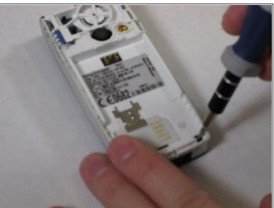
Remove the four screws located at each corner of the device.
