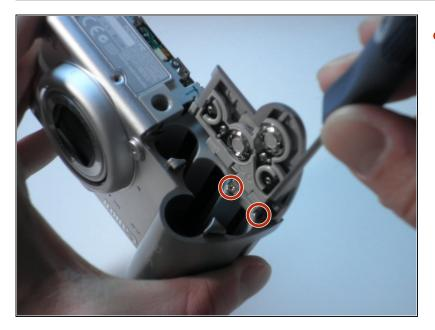
• Remove the two screws at the top of the battery compartment with a Phillips #00 screwdriver.
