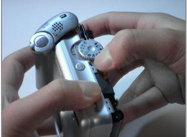
• With your right thumb, pull back on the tab while using your left hand to pull the face of the camera away from the body.
