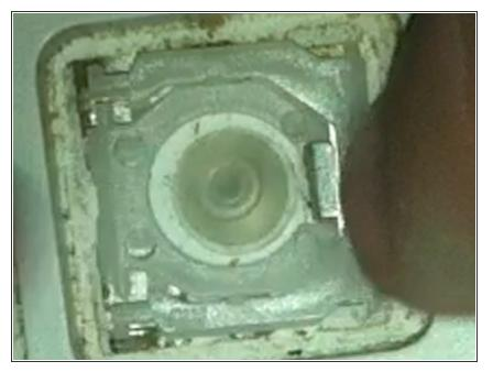
Now what you want to do, is hold the mechanism flat side up. Put the mechanism into the hook on the right side. A spudger or small flathead might help.
