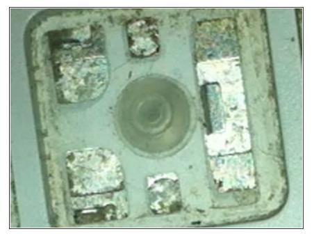
Once you have removed and cleaned the key (or have not cleaned) take a close look at the key. There is a big hook on the right side, and two smaller hooks on the top left and bottom left.
