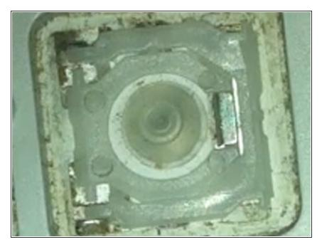
Now pop in the two pins on the bottom left and top left into their hooks using a small spudger or flathead.
