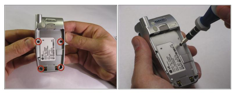
Use a Torx T6 screwdriver to unscrew the four screws on the back of the phone.
