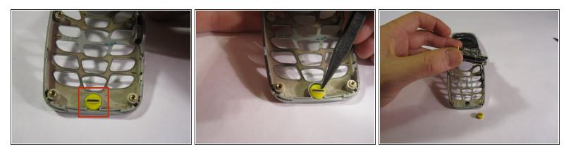
Using your fingers or the pointed end of a black plastic spudger, pry the microphone out and replace.
