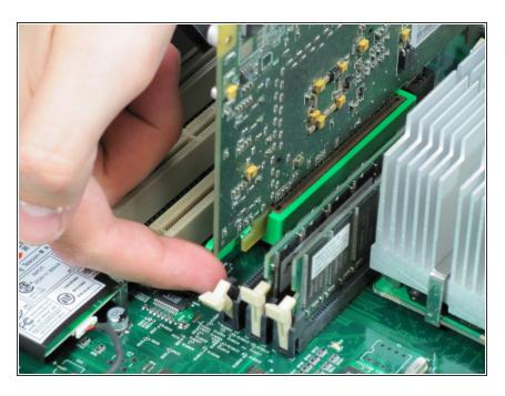
Before lifting the card out, this small plastic tab needs to be pulled back there by releasing it entirely.
