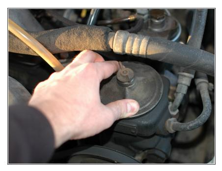
As the nut loosens use a second hand to hold the cover down. There is a spring under the cover that will force it up and make it harder to remove the retaining nut.
