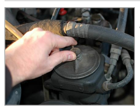
To remove the cover begin by loosening the retaining nut. On this car it is a metal wing nut, but on some W123's there is a plastic thumb nut.
