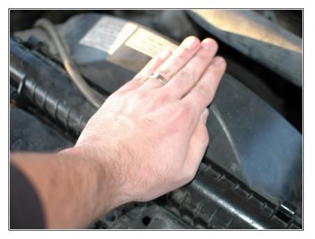
Once you have verified that the coolant is cool enough to proceed, use the palm of your hand to press down on the radiator cap and turn it counter clockwise.
