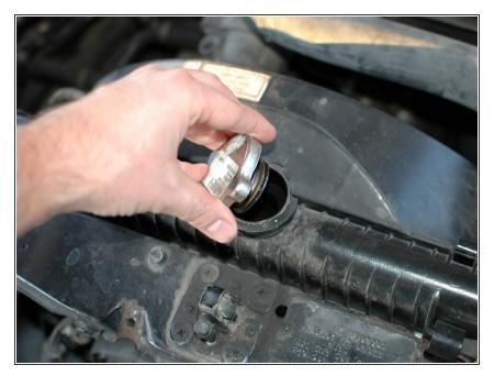
• Pull the cap up and out of the radiator and set it aside.
