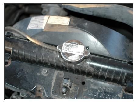
Make sure the cap is fully tightened. After your next drive check the cap for leaks and tighten further if necessary.
