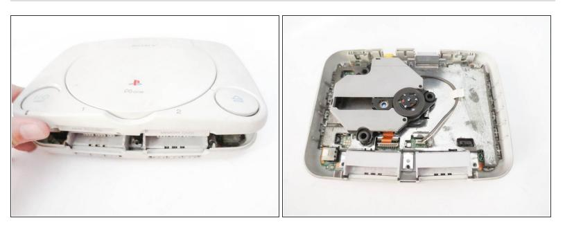
• Lift up and remove the upper case.
