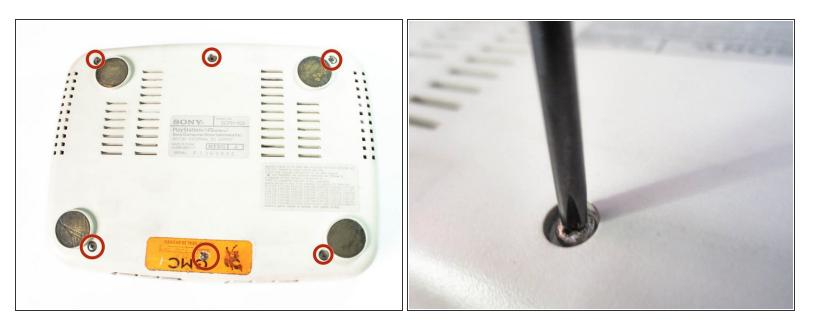
Flip over the PlayStation and remove the six screws from the bottom.
