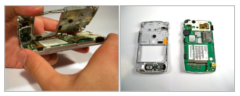
• Gently lift and remove the back casing.
