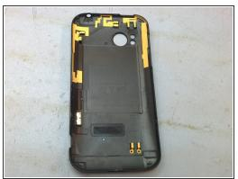
Remove rear cover using little notch located at bottom of phone
