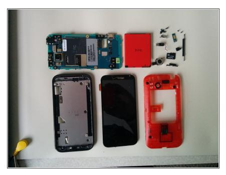
For the most part, this teardown is pretty straightforward with the headphone jack fused to main board. The display looks to be fused to the screen so replacement of either means replacement of both.
