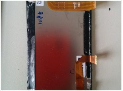
Using pick or pry tool, slowly remove screen from frame. Tape and adhesive is holding it on so work slowly and use heat gun if needed.
