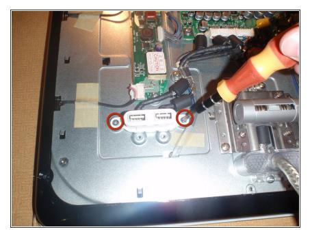
Remove the two phillips head screws on the sides of USB port, using #2 phillips head screwdriver.
