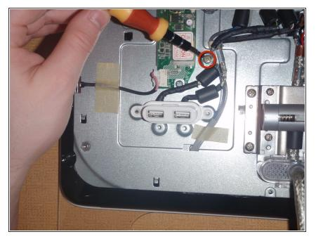
Remove the single screw on the cable hold-down, using #2 phillips head screwdriver.
