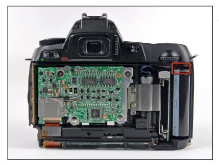
⚠ At this point, the capacitor is visible and its exposed contacts are boxed in red. Even though they are recessed, be careful not to touch the contacts to avoid shocking yourself.
