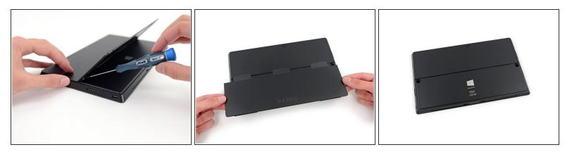
Remove the two T5 Torx screws, then take off the kickstand.
