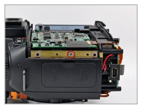
Remove the 3.8 mm silver Phillips screw securing the port cover to the side of the D70.
