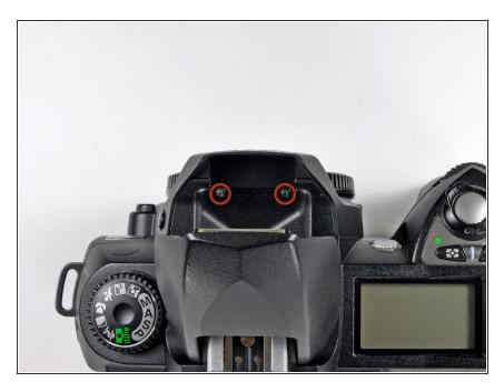
Remove the two 4.3 mm Phillips screws securing the top edge of the front cover to the top cover.
