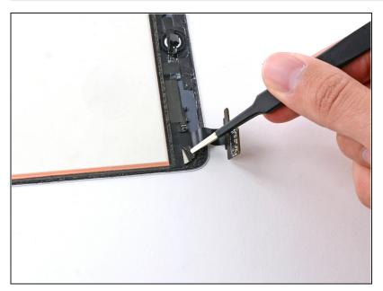
i If necessary, use a pair of tweezers to partially peel back the piece of tape covering the smart cover magnet near the lower left corner of the front panel assembly.
