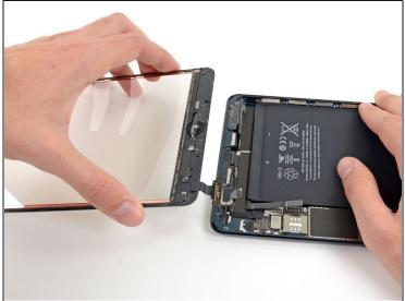
• Lift and remove the front panel from the iPad.
