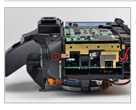
Remove the Phillips screw securing the top cover to the D70 near the mode dial.
