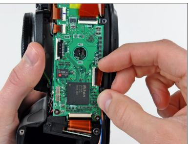
Use your fingernail to flip up the ZIF locking flap on the LCD ribbon cable socket.
