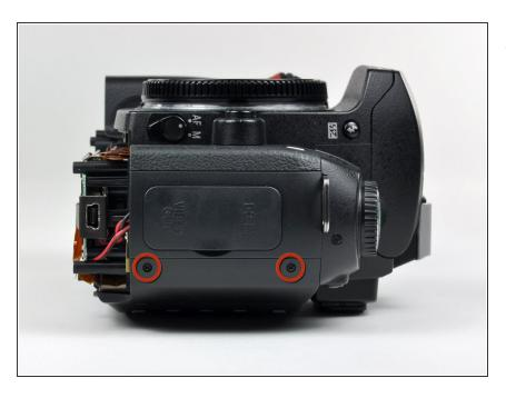
Remove the two 4.8 mm Phillips screws securing the port side of the rear cover to the D70.
