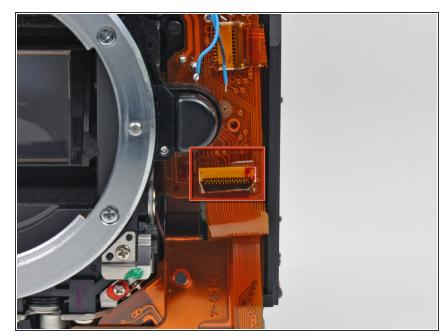
if present, remove the piece of tape covering the ribbon cable socket (boxed in red).
