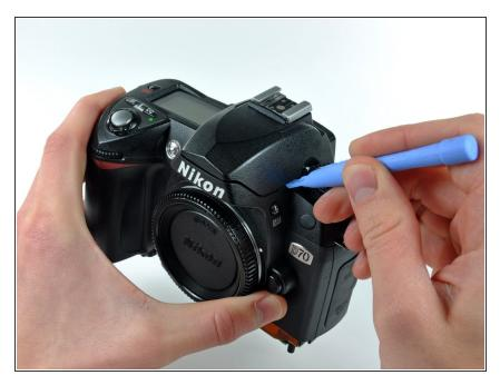
Use a plastic opening tool to carefully pry up the flash unit at the point shown in the picture.
