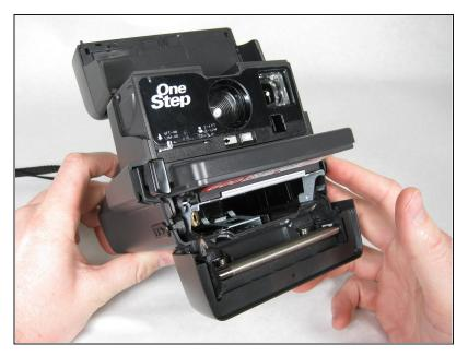
• Open the battery/ cartridge compartment fully.
