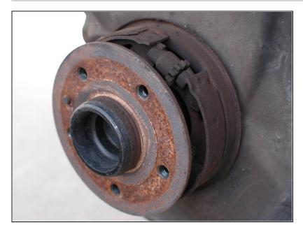
With the rotor off the rear hub is exposed. It may be quite rusty like this. If the rotor was seized to the hub it was because of this rust.
