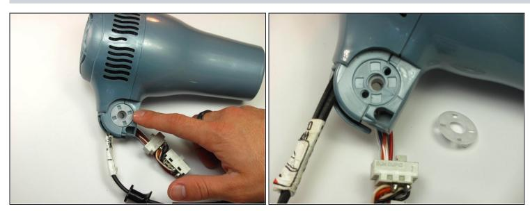
• Remove the inner white disk piece from the base of the dryer head by gently pulling it out with your finger nail.
