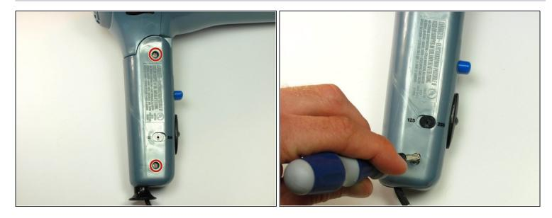
Unscrew the two 18 mm long Phillips #2 screws on the side of the hair dryer.
