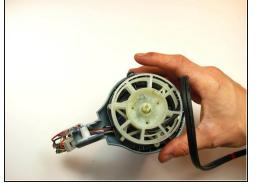
Once the coil is removed, unscrew the three 11 mm long Phillips #2 screws underneath to remove the retracting wheel.
