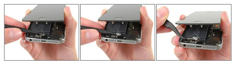
• Open the phone just enough to reveal the metal bracket covering the home button cable.
