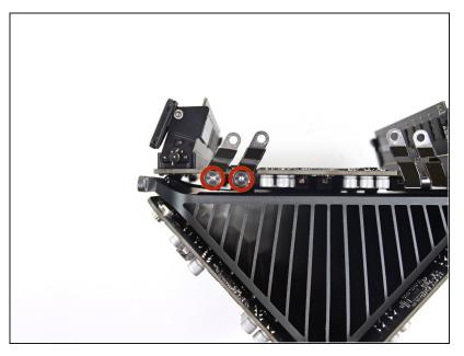
• Remove two 5.5 mm T8 Torx screws.
