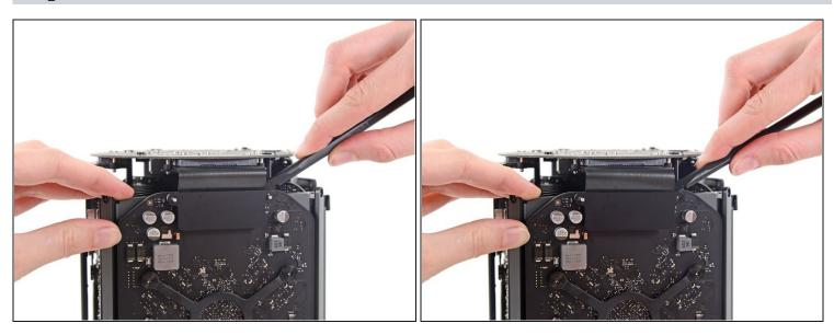
• Use the flat end of a spudger and a twisting motion to gently separate one side of the graphics card data connection.
