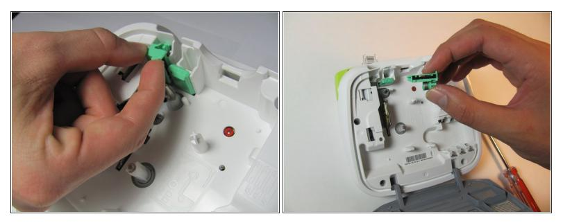
Using the thumb and forefinger, pull up, applying a moderate amount of pressure until the cutter blade unit loosens and is removed.
