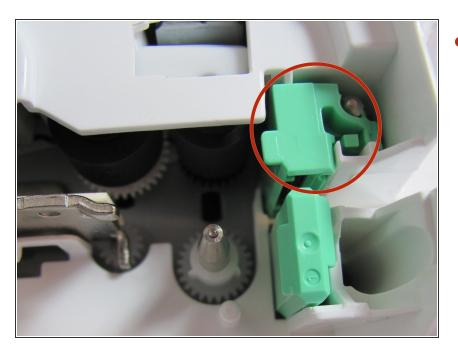
• Locate the cutter blade unit (mint green) as shown in the picture.
