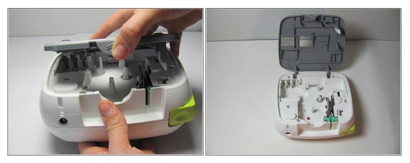
• Open the back panel of the device by pressing down on and then pulling the indication arrows on the top center of the cover upward towards you.
