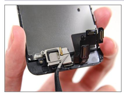
• Remove the bracket from the display.
