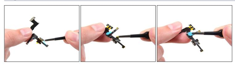
• Remove any clear backing strips from the light sensor, cable and front-facing camera.
