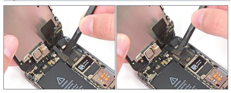
• Finally, disconnect the digitizer cable connector.
