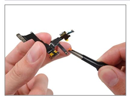
Remove any plastic coverings from the microphone on the sensor cable assembly.
