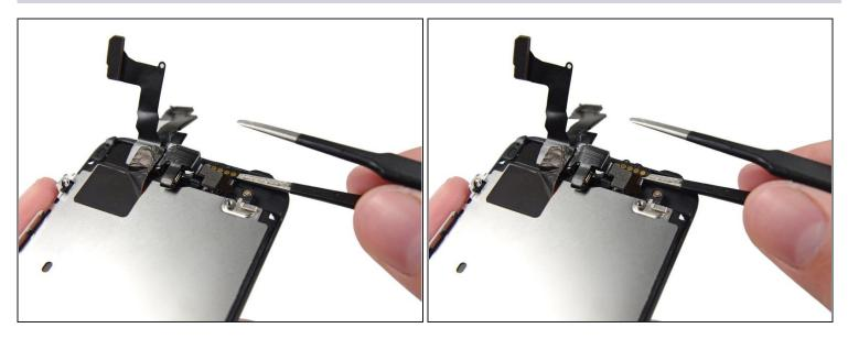
• Using the edge of a set of <u>tweezers</u> or a metal spudger, gently pry the earpiece speaker contact cable up, to separate this portion of the camera and sensor cable from the adhesive below.
