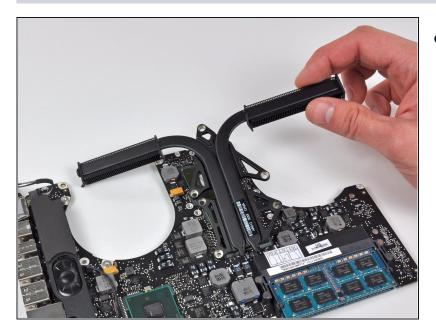
• The heat sinks can be separated from the logic board, leaving it very cold and lonely.
