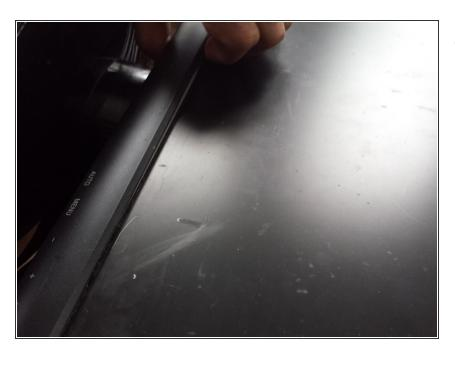
Remove front bezel by lifting softly starting from the middle and moving out to the corners.
