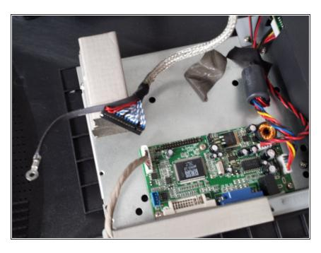
Remove the data connector and ground.
