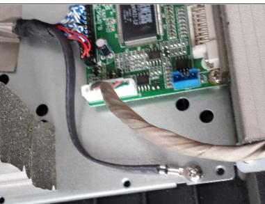
After removing the connectors, slide it about 3-5 inches to the right to have access to the data connector and ground
