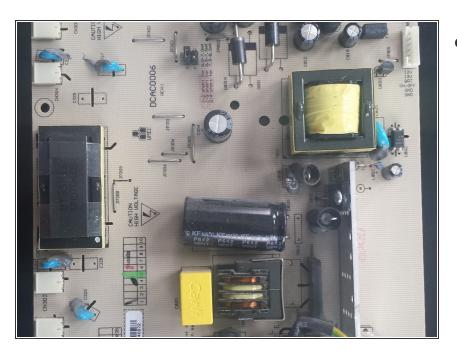
Power board displaying the capacitors to be replaced
