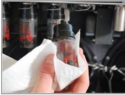
Using the cloth, you can then remove a tube by pressing up on the two metal flaps near the top of the tubes, while lightly pulling the tube down.
