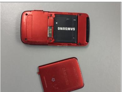
Remove the battery cover by pushing it upwards.
