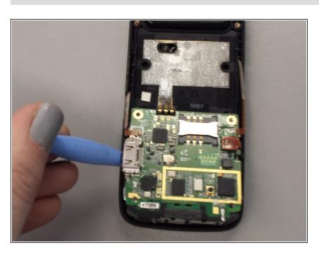
Use the small plastic opening tool to gently remove the motherboard from the rest of the phone.
