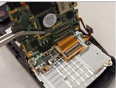
Gently grab the motherboard with tweezers, then disconnect it from the two attached plates.
