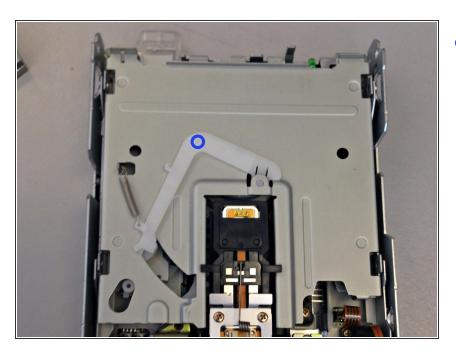
Flip the device over so the plastic arm is face up.
