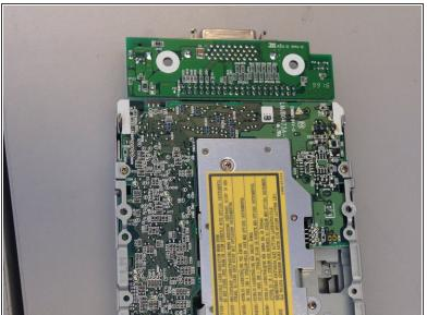
Slide disk drive out of metal casing.
