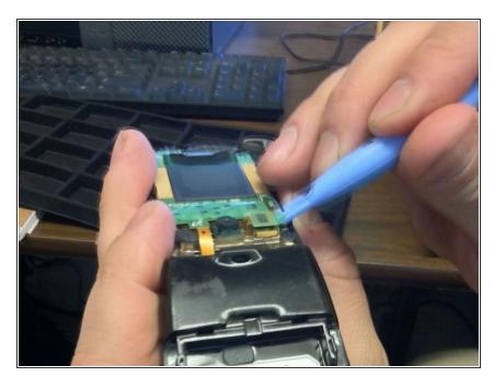
Using a plastic opening tool, disconnect the electrical connector.
