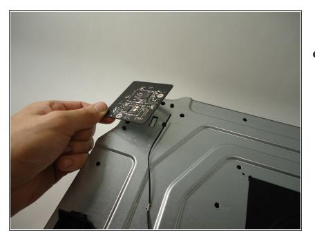
Carefully pull the Wi-Fi board straight up to release it from the chassis. The Wi-Fi board is now free.
