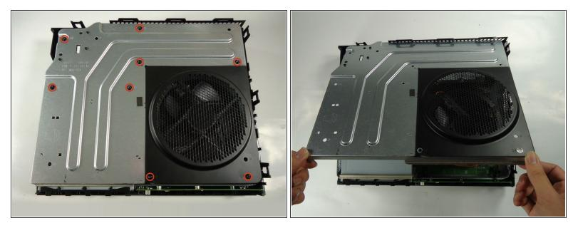
Remove all eight of the 64.0 mm, T-9 screws labeled C1 through C8 securing the chassis top to the motherboard.
