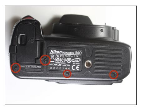
Remove the four highlighted 3.0 mm
