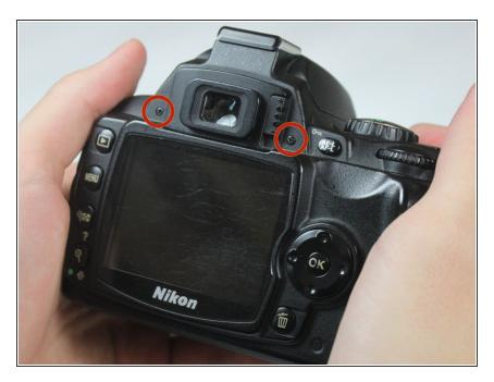
Remove the two visible 6.0 mm
