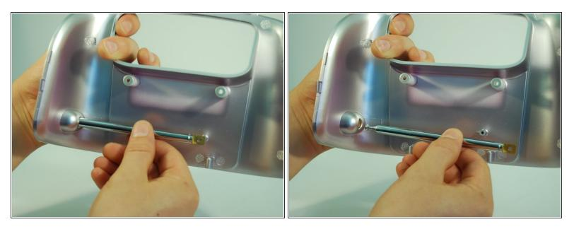
• If desired, the antenna can now be removed by pulling **inwards** and horizontal to the panel bottom.
