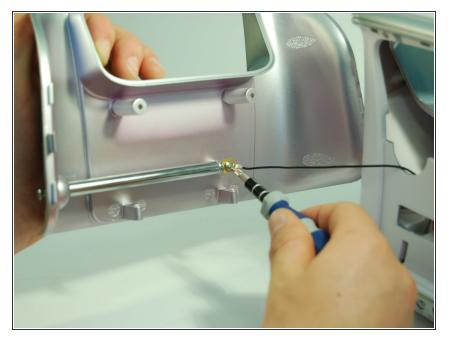
Use a Phillips #1 screwdriver to detach the wire from the back panel by removing the 8 mm screw connecting the wire to the antenna.
