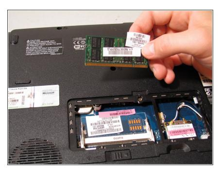
Slide the RAM out of its position and remove it.
