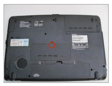
Unscrew the 4mm screw from the middle panel using a Phillips #1.
