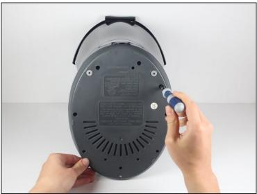
• Remove the eight 11 mm screws that secure the base of the machine with a Phillips Head #2 screwdriver.
