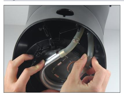
Once the crimps are loosened, slide them down the tubing.
