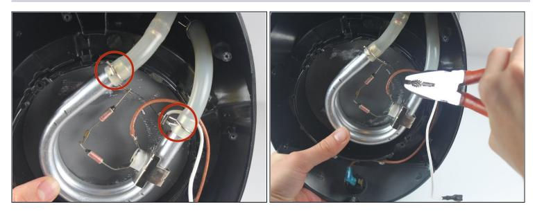
Use needle-nose pilers to pinch and loosen the crimps
