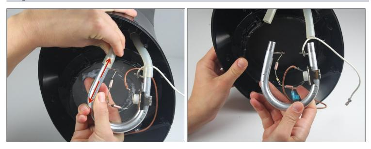
• Separate the tubing from the heating coil by grasping the tubing in one hand and the heating coil in the other and gently pulling apart.
