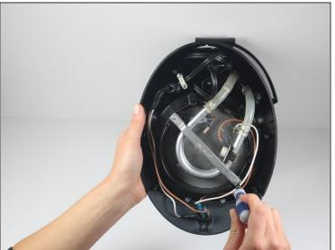
• Remove the two 13mm screws securing the silver support bracket using a #2 Phillips head screwdriver.
