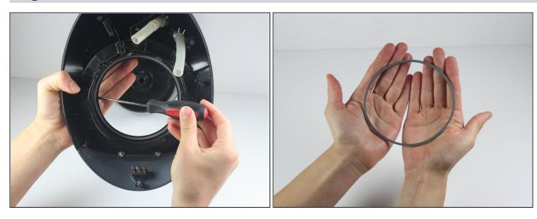
• Use a <u>2.5 mm Flathead</u> Screwdriver to pry out the O-ring.
