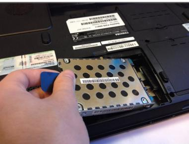
Hold the black tab attached to the hard drive and pull with medium force to the side that the tab is on. This will pull the hard drive out of it's socket.
