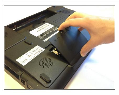
Place one finger under the tab of the hard drive panel and lift up with medium force.
