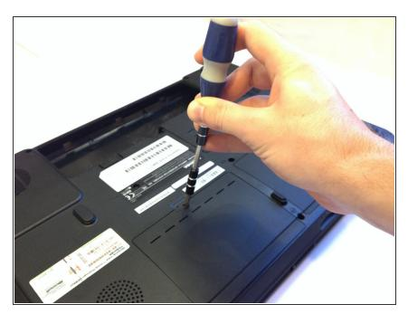
Use a #1 Phillips screwdriver to take out the 8mm Phillips #1 screw holding the hard drive panel on.
