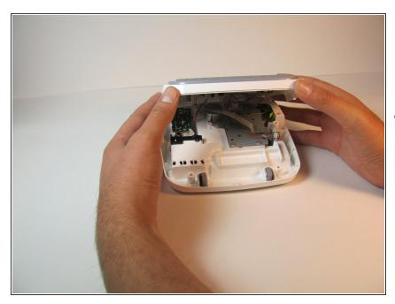
• Close the back cover and then flip the device over and separate the top half from the bottom half as shown.
