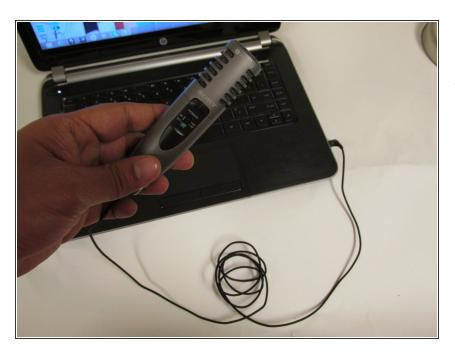
Some volume issues could be related to other external devices, such as a laptop. This particular microphone was not designed to be used with a computer.
