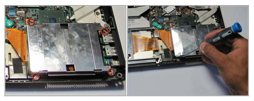
Remove the screws holding the hard drive casing in place.
