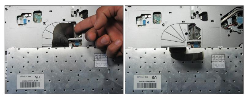
• Lift up lever underneath the ribbon to detach the keyboard.
