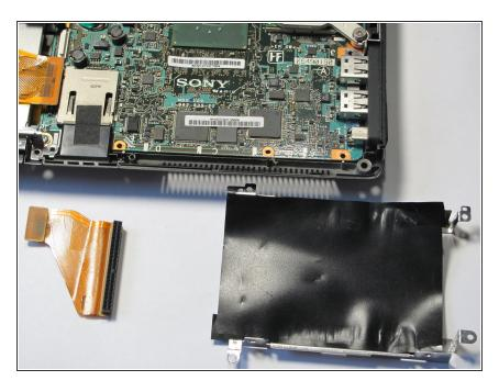
• Remove the casing and the orange ribbon.
